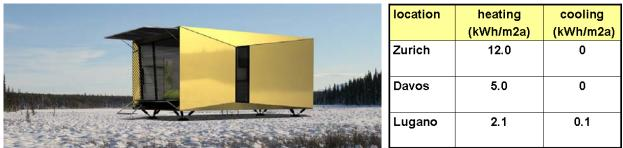
Outline sketch of the space unit "satellite" (left) and heating and cooling requirement for 3 locations (right).
