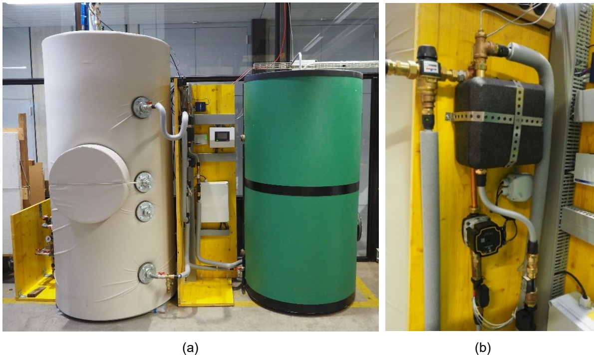
Figure 56: Storages and heat transfer with a) solar drainback storage (grey) and DHW storage (green) and b) components for heat transfer and system control between the storages (passive thermostat, plate heat exchanger, pump, and flow detection sensor)..
