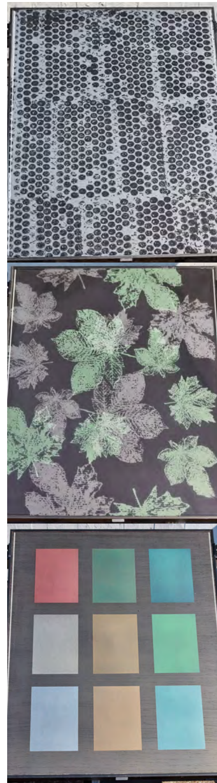
Figure 3: Standard CI(G)S PV modules after treatment of glass cover with sandblasting techniques (top) and sandblasting & colouring techniques (centre, bottom) [6], [7].
