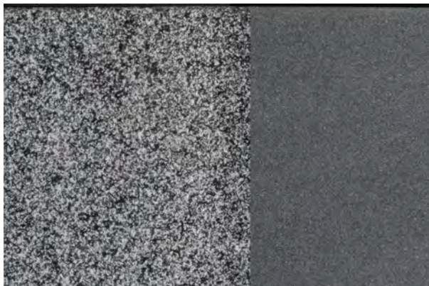
Figure 2: Close-up of two sandblasted glass specimens with different grain-sizes blasted for laboratory measurement.
