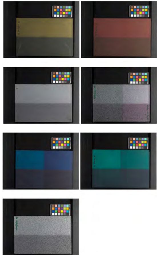
Figure 5: Sandblasted and coloured glass specimens. The pictures show a selection of the test specimens with black and white back-layers.
