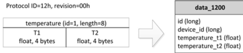
Figure 5: An example of the mapping of a data channel to the database table
