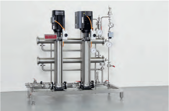
Figure 3 Skid mounted nanofiltration unit for de-alcoholisation of 50 hl/d beer
