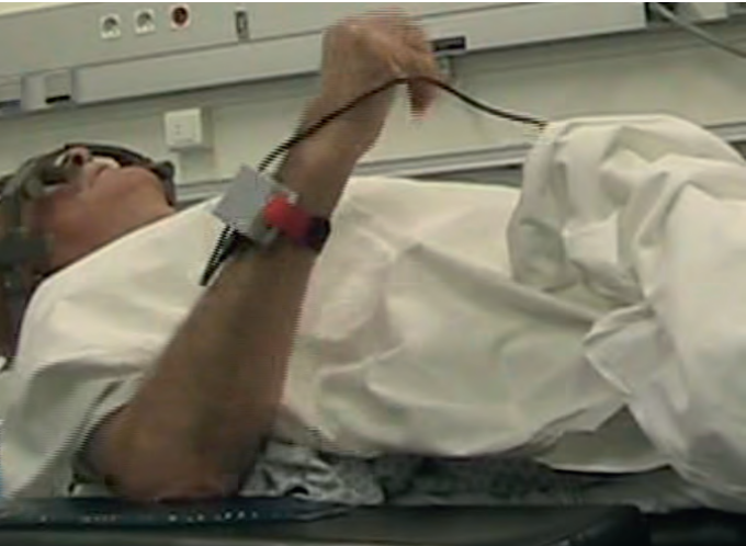
Figure 1 Accelerometer tied to the patient's wrist for evaluation of tremor.
