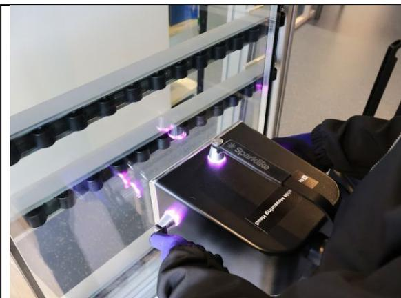
Abbildung 10: Sparklike Laser Portable Sensor ©Sparklike [12]
