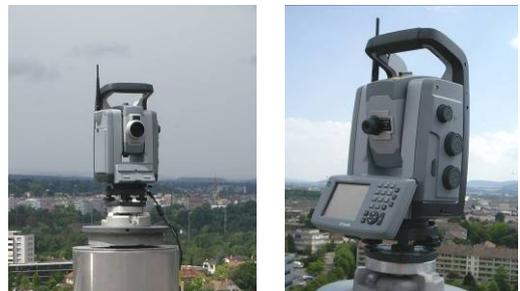
Abb. 2: Totalstation Trimble S8
