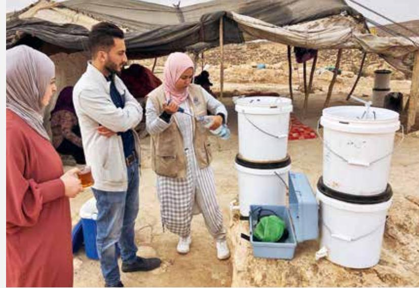
The researchers tested three ceramic filters and two membrane filters – 150 filters each in Kenya and the West Bank and 120 in Somalia. Every family that wanted to could take part and the filter type was assigned at random. A special feature of the study was that each household was allowed to test a second filter after the first four months. Peter explains: “Many needy people in developing countries do not dare criticise any-
