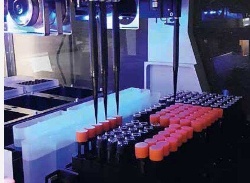
says Germershaus. "It is about one and a half times faster than humans, can produce the formulations very reliably and does exactly what it was programmed for. In addition, the robot has a clean-air hood to filter the air and remove particles and microorganisms, enabling it to produce the formulations under sterile conditions."
