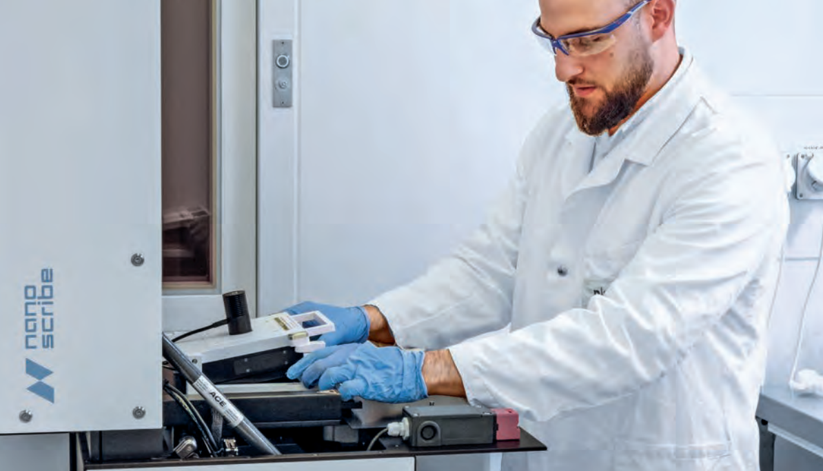
PhD student Ilias Amara produces artificial reference particles using two photo polymerisation.
