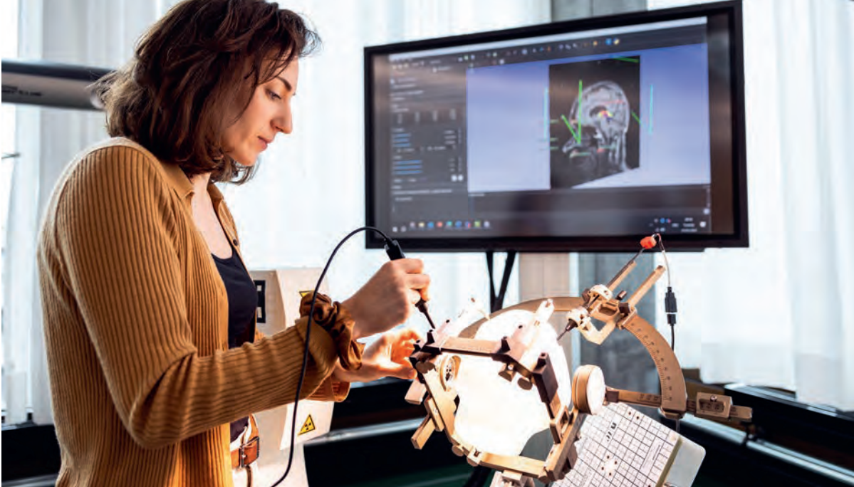
Céline Vergne tests her electromagnetic navigation system for localisation of electrodes in the brain, using a head phantom inside a stereotactic headset.
