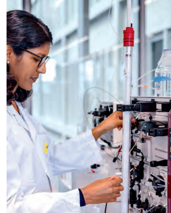
Doctoral researcher Sherin Panikulam performs chromatography to purify biologics, and analyses whether host cell proteins remain after purification.
