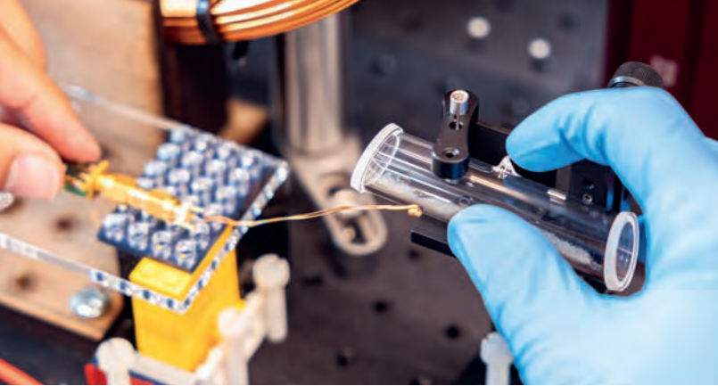
Atomic vapor cells can be used to measure tiny magnetic fields such as the one emitted by the human heart.
