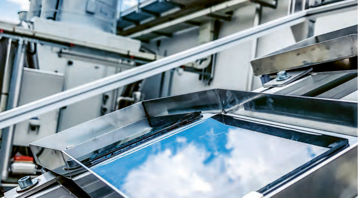
Lenz’s team conducts outdoor leaching tests to assess the safety of perovskite photovoltaic panels installed on the roof of the FHNW Campus in Muttentz.
